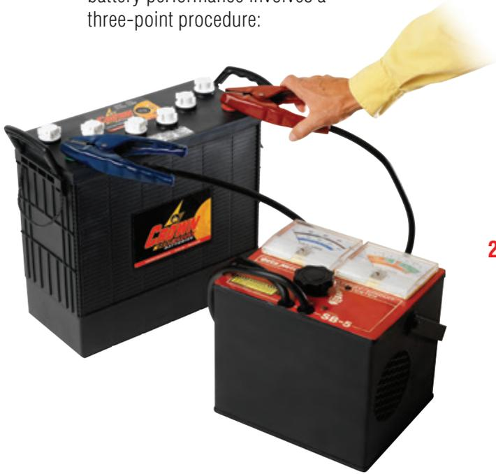
**1. Visual Inspection:** Check battery age or length of service if available. Inspect battery for damage - when physical damage to the battery container or terminals is present, replace the battery. If none, check the battery's cell electrolyte levels. Fluid levels should be above the top of plates in all cells, and no higher than the top of the fluid level indicator:
