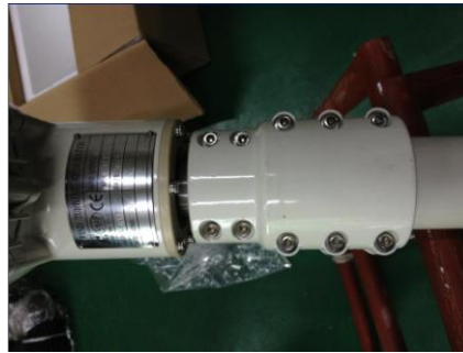
⑤ The pole is inserted into lower part of the clamp.
