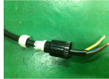
③ Pass the wires through the cover.
