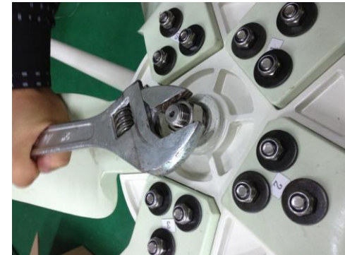
③ Fully tighten the nut to 154N.m
