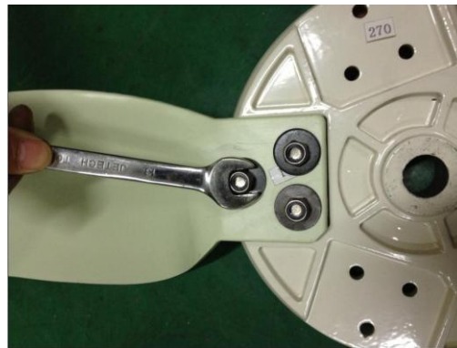
⑤ Place blade, flat washer and nylock nut, and tighten the nut to 18N.m
