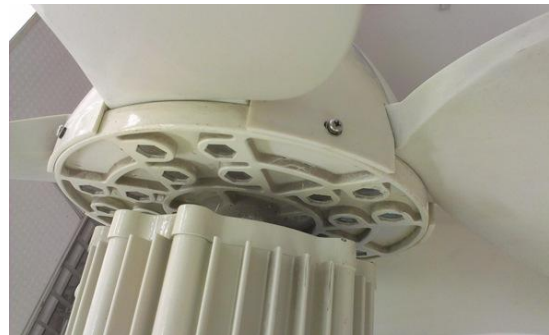
⑤ After installation tug on the nosecone to make sure it is securely attached and turn the blades to make sure it is not rubbing against the front cover of the generator.
