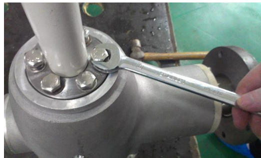
⑤ Tighten the bolt to 35N.m
