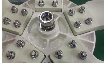
② Place the hub with blades onto the rotor shaft and “spin” it completely onto the turbine alternator shaft, then place in sequence of flat washer, spring washer and nut.
