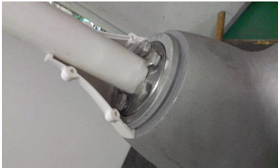
⑦ Snap the cover to the back of generator
