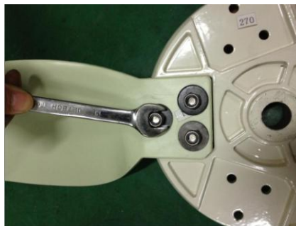
⑤ Place blade, flat washer and locknut, and tighten the nut to 30N.m
