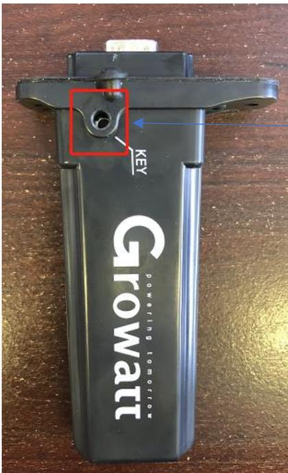
Open the rubber cap and find KEY hole, both LED indicator and reset button are inside of it.
