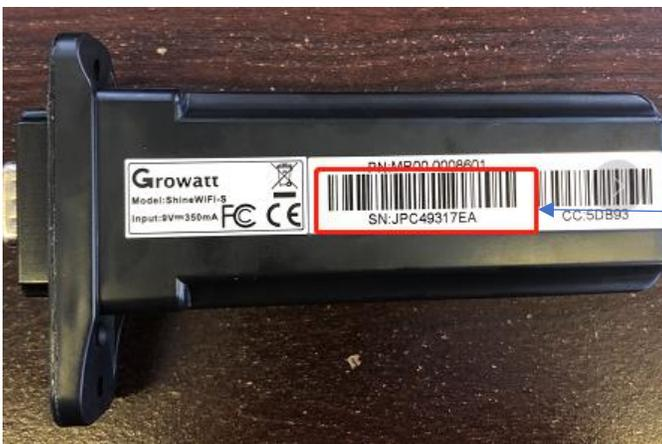
The bar code is on the back of the dongle, where the serial number and the check code can be found.
