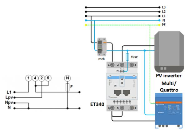
On the GX device go to the grid meter in the Wired AC sensor settings. Make sure 'Phase type' is set to 'Single phase' and 'PV inverter on phase 2' is enabled.
